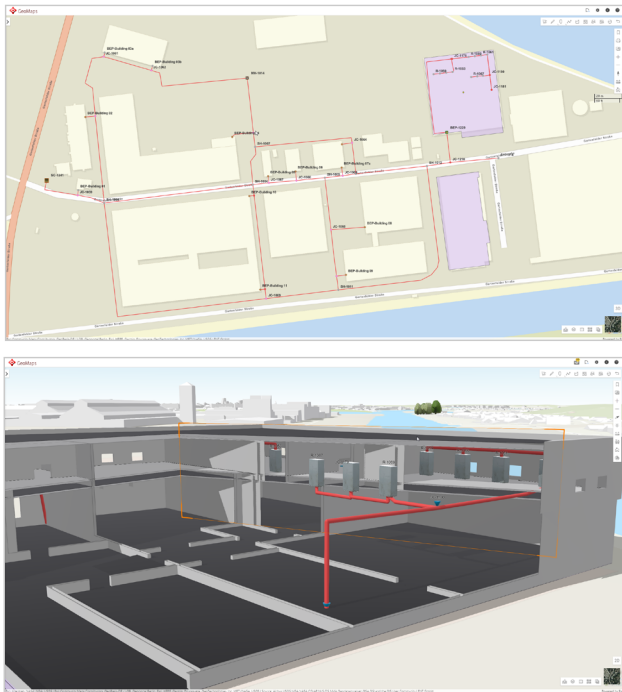
A GIS application provides transparency into assets and resources in cable networks: infrastructure objects are not only shown georeferenced on maps, the details go down to the level of floors and rooms
